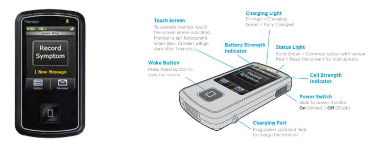
**The MCOTos Monitor** is a small portable device that gathers data from the sensor and sends the information to our 24 hour monitoring center. The monitor automatically transmits data using a built-in cell phone. Although the monitor will transmit ECG's from your heart automatically, it is important to record symptoms as you feel them. This will provide additional information on the reports received by your physician.
