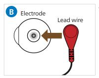
Snap each lead wire onto an electrode.
